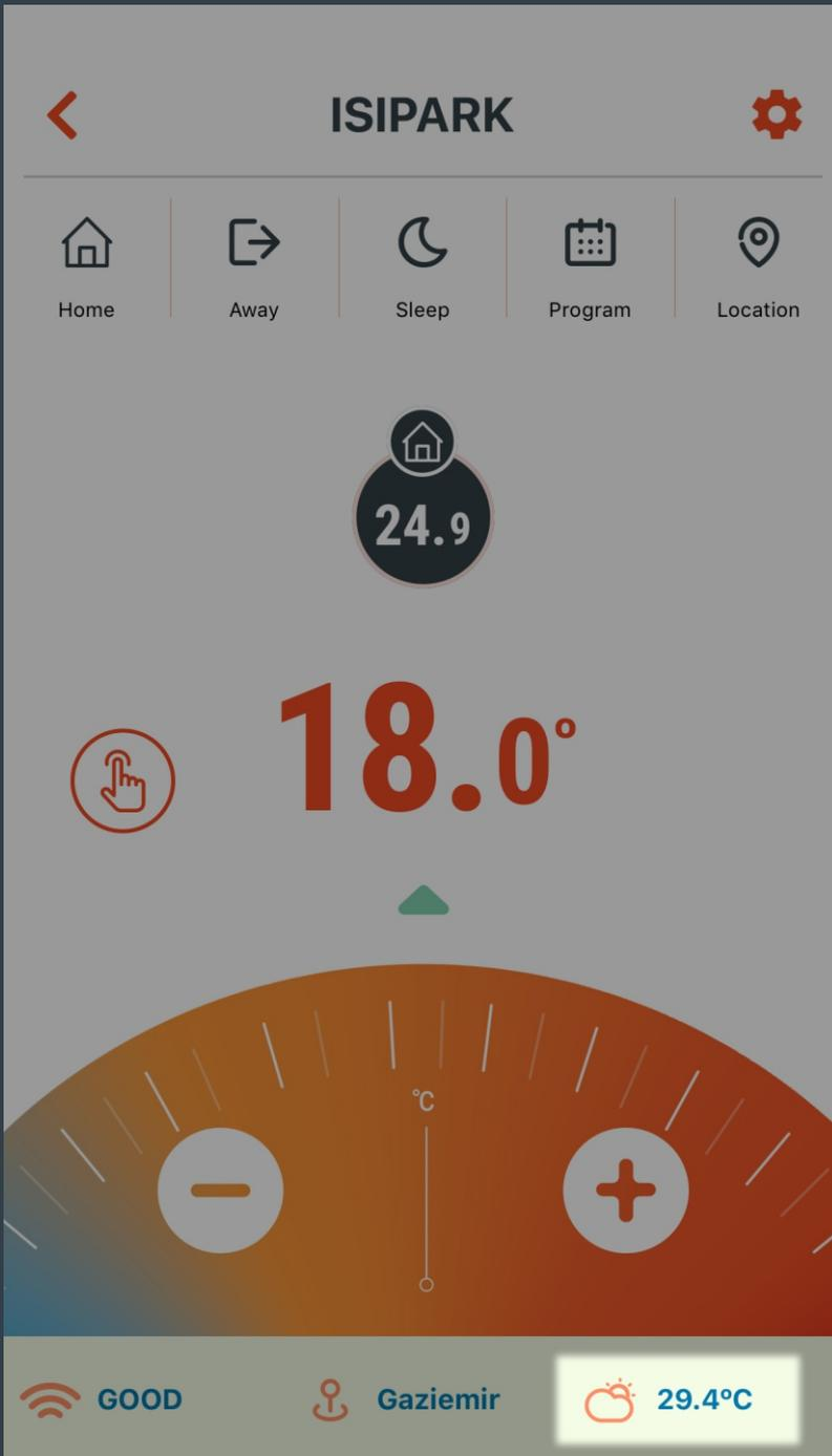
Estimated outside temperature taken from the meteorological data station according to the position of the HT400 is shown here.
