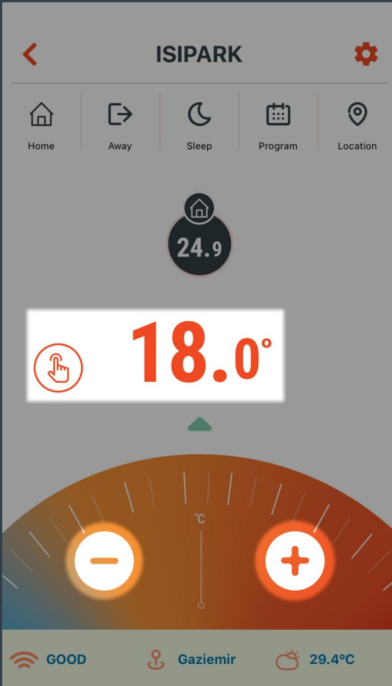
⊖ button reduces the set temperature value and the heating unit is managed according to this value.
