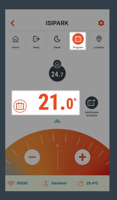
The heating unit is managed according to the temperature in the schedule added on a day and 30 minute basis in the Program Mode.
