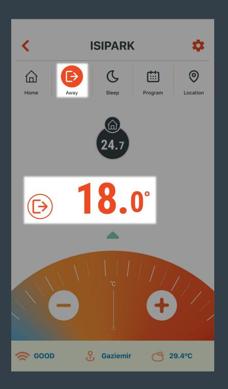
The heating unit is managed according to the temperature set for away mode.
