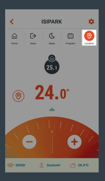
Press the "Location Mode" button for 3 seconds to quickly switch to the "Location Mode" settings.
