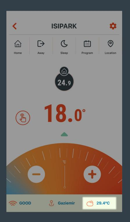
Estimated outside temperature taken from the meteorological data station according to the position of the HT300S SMART is shown here.
