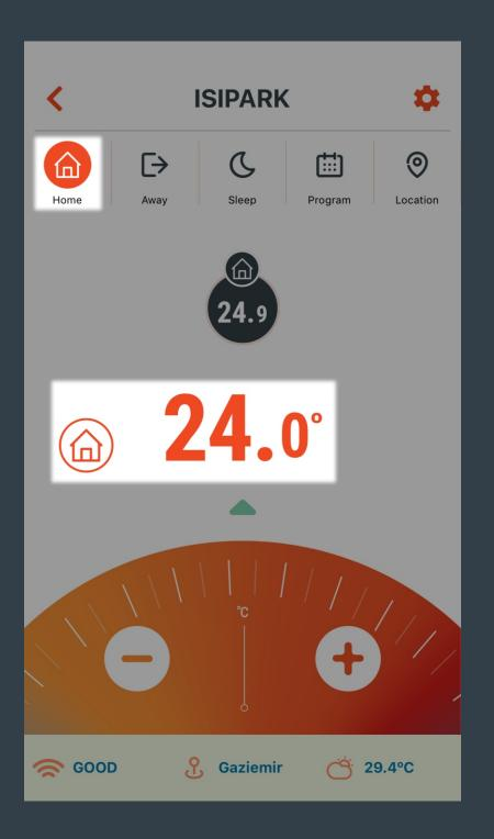
The heating unit is managed according to the temperature set for home mode.
